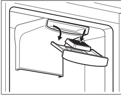
3. Insert the new air filter in the slot.
