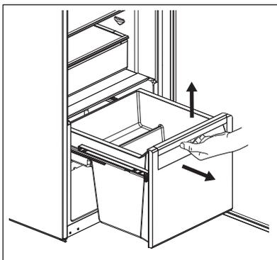
2. Push the rails inside the cabinet to avoid damage to the appliance when closing the door.
